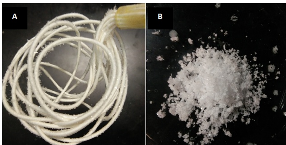
Fig. 3. NaCl crystals formed (A) on the membrane surface and (B) in the bulk solution.
